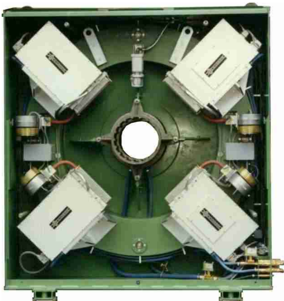
2 axis gauge DO 300/2 measurement field 300 mm
