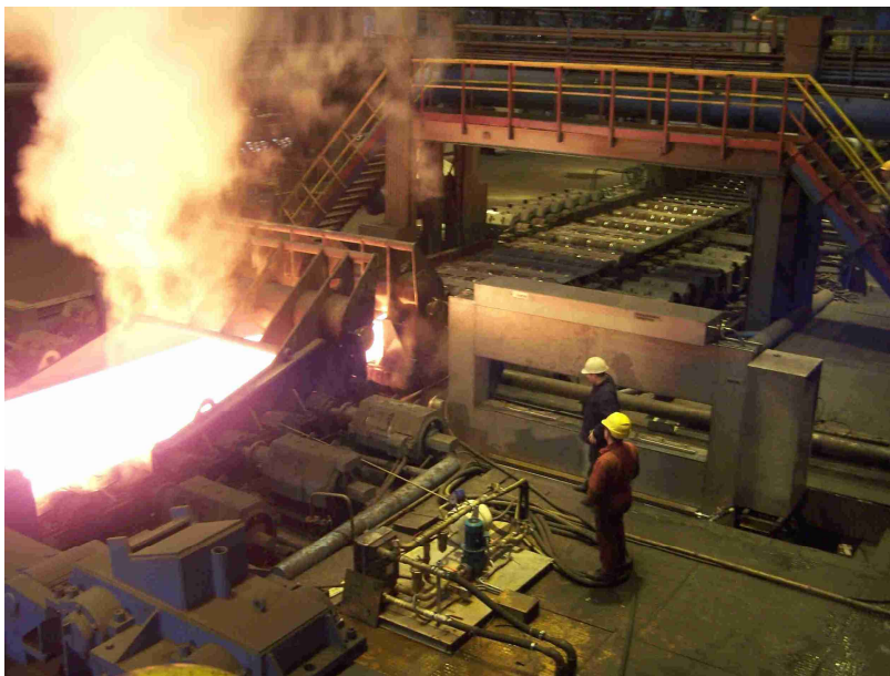
LASER gauge AMK 2800 for measurement of thickness (5-50 mm) and width (1500-2800 mm) of sheets in a hot rolling mill
