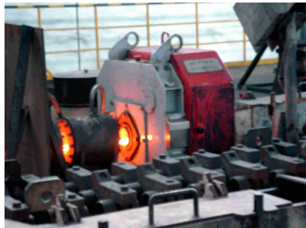
DO 75 RO-D in a bar mill measurement field 75 mm 8 entire profil measurements/s
