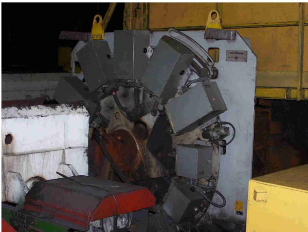
6 axis gauge DO 200/6 in a hot mill measurement field 200 mm
