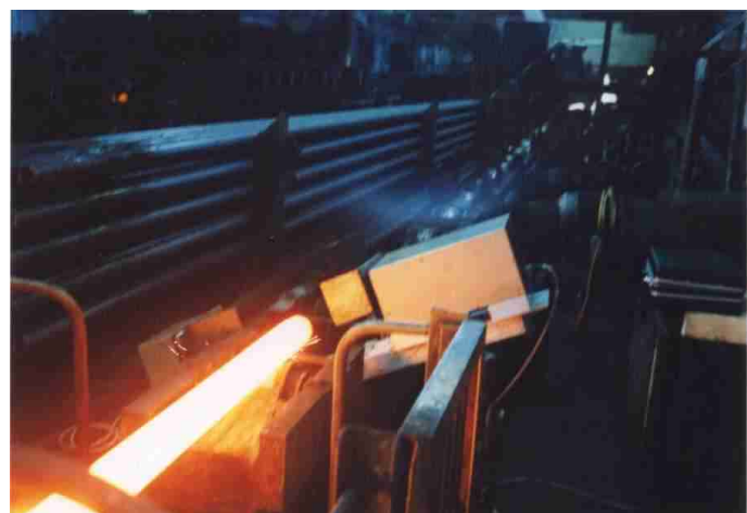
1 axis gauge for measurement of mandrels measurement field 200 mm
