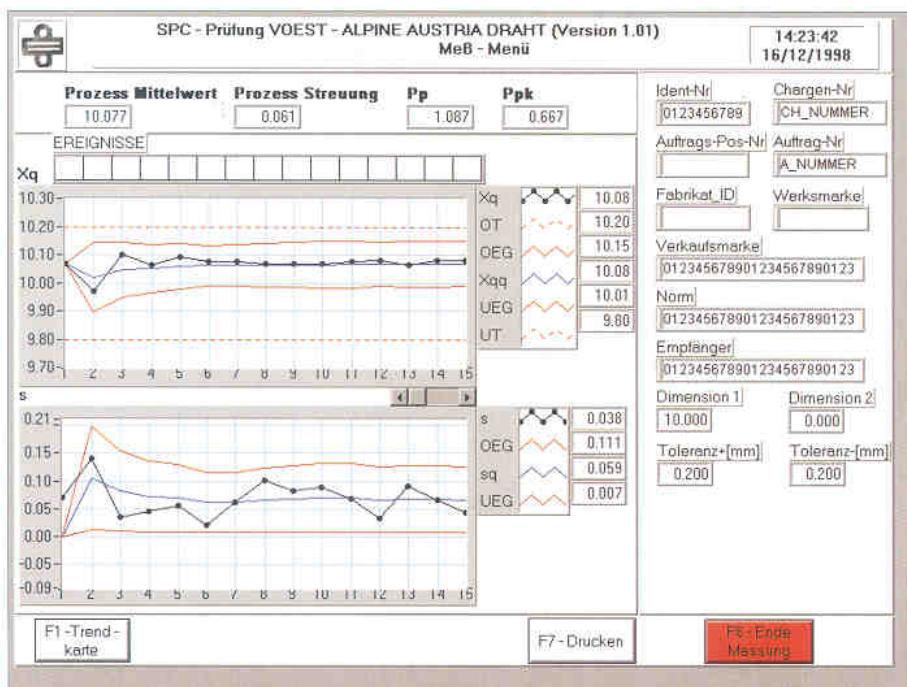
The QS-Line SPC corresponds to ISO 9000 QS-standard. The structure of the QS-Line SPC is designed for easy adaption to the customer's specific requirements.
